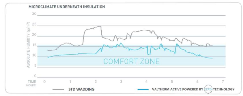
Insulation system with 37.5 technology (blue line) was in the comfort zone 97% of the time, whereas in the system without 37.5 technology (grey line) the user was in the comfort zone only 23% of the time.
